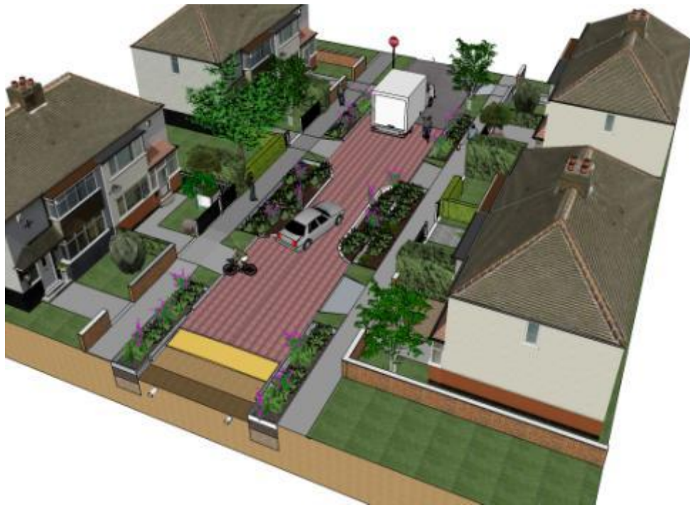
Figure 11-4 Permeable paving and road side rain gardens
