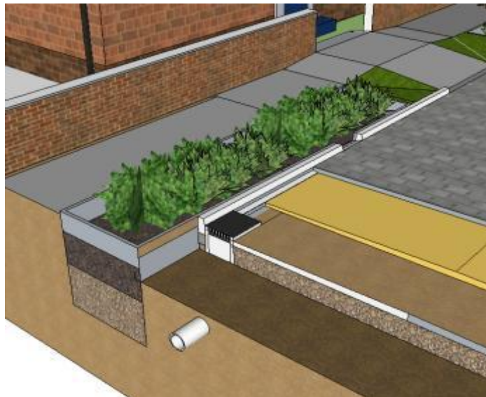
Figure 11-5 Typical example of a road side rain garden
