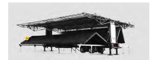
SL320 stage arrives on a lorry and unfolds
