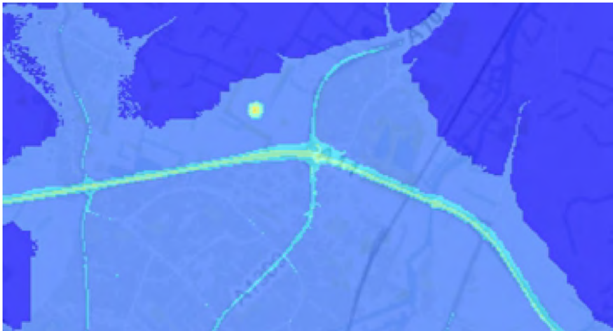
Figure 8: Annual Mean PM 2.5 Concentrations, µg/m 3 (based on existing NAQO of 25µg/m 3 , respectively)
