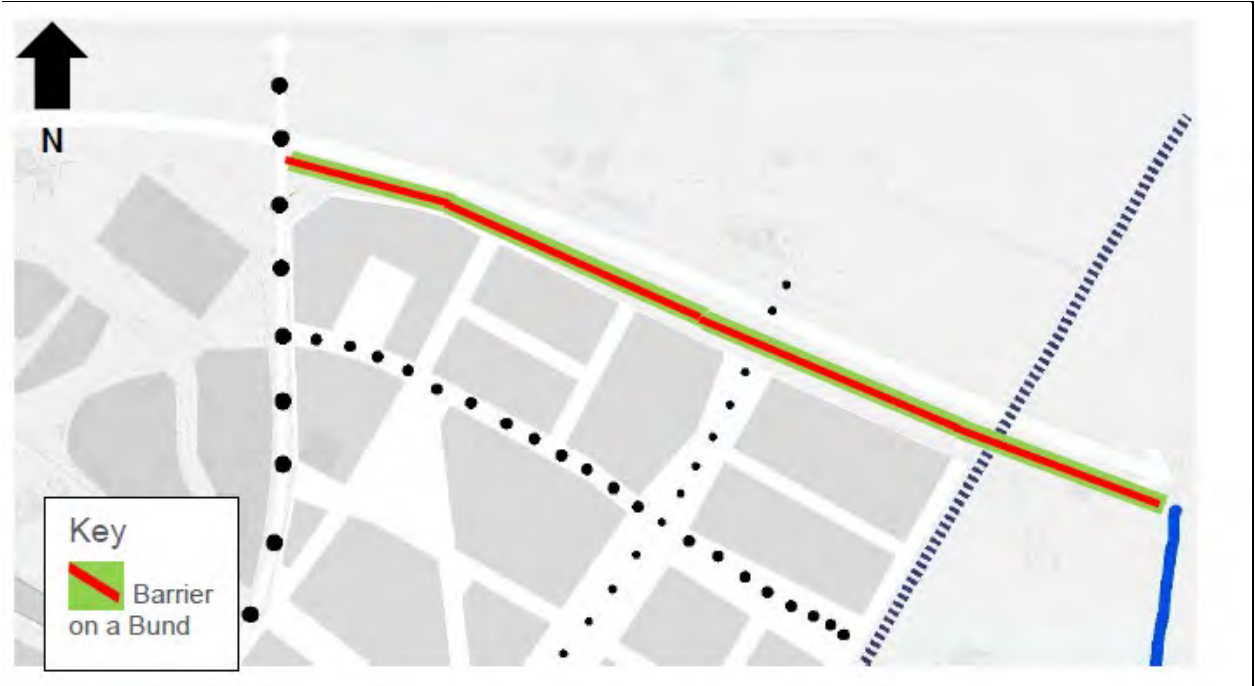
Figure 3-9: Suggested Location of the 3m or 4m high Barrier on a 3m High Bund
