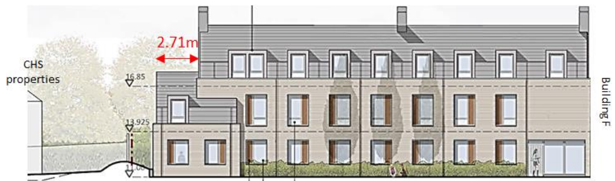
Front view of Building F shows lower section is 2.71m wide
