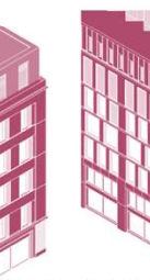
3.6.5 First level of double plant expressed as part of the primary facade, where glazing appears solid
