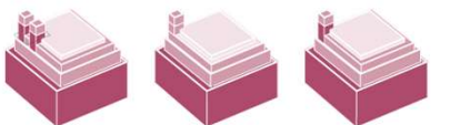
3.7.5 Flues integrated with the architectural strategy - grouping of two flues 3.7.6 Flues integrated with the architectural strategy - with plant screen materiality 3.7.7 Flues integrated with the architectural strategy - with primary facade material
