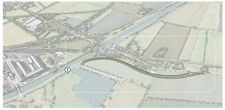
**Option 1 South East highway** – A new highway, of approximately 900 metres, connecting the B1382 to Queen Adelaide Way, would provide a new route for through-traffic towards Ely and the southern bypass and reduce traffic running through Queen Adelaide and across the level crossings. The existing three level crossings would be upgraded to full barriers to manage the safety risk to users from the additional rail traffic.
