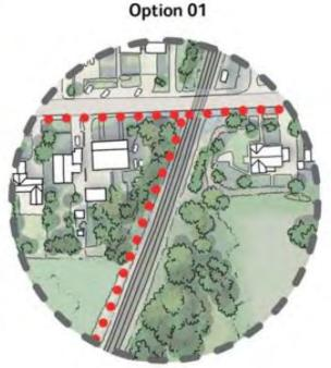
**Option 1** – divert footpath along the western side of the Peterborough line to link with Ely Road. This may require the compulsory purchase of land to enable a new footpath of two metres wide to be installed.
