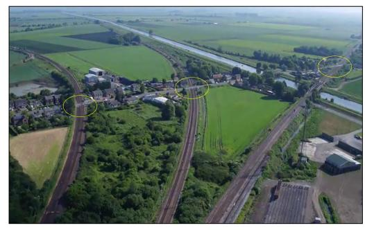
To the north east of Ely, there are three level crossings within the village of Queen Adelaide on the B1382 (Ely Road) in close proximity to each other which poses a significant challenge to increasing capacity while maintaining the road connection into Ely.
