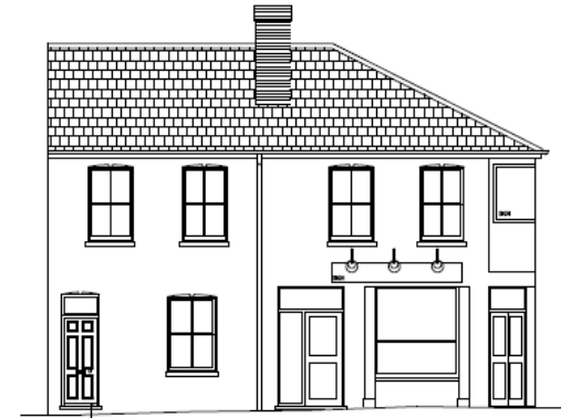
Elevation B-B Scale 1:50 Existing door retained with new wall behind it - fanlight retained
