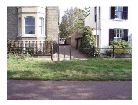
Remove bollards and replace with a pedestrian gate. Put in a tarmac path link.
