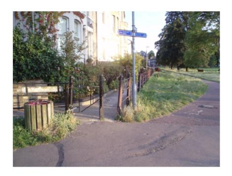
Reconfigure bollards with larger gate to achieve 1.0m (this distance is the width of all other entrances with cattle grids leading onto the common). Monitor for any problems.
